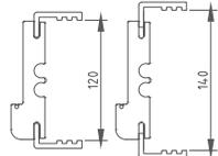
ESPESOR MÁXIMO DE MURO AJUSTABLE DE 120 MM A 140 MM
